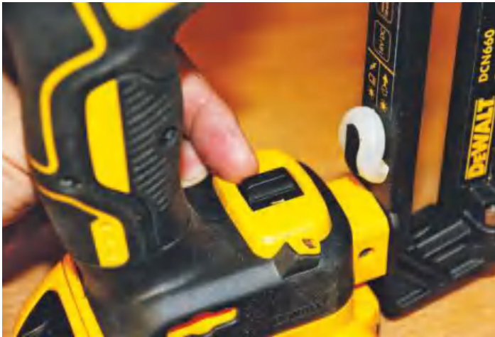
▲ A second switch alters the tool from sequential to bump mode
